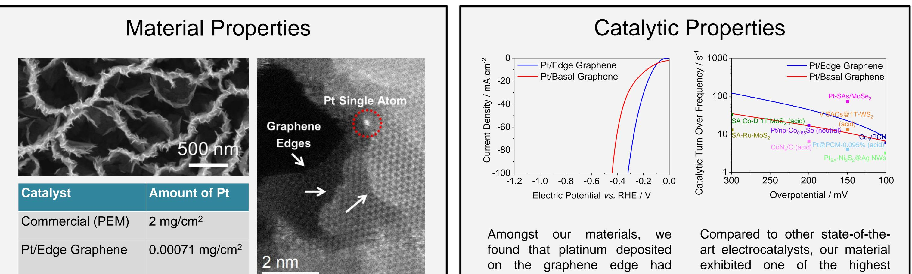
Electron microscopy revealed that the platinum deposited was in single atom form, decorating the graphene edges. These single atoms are the sites where hydrogen is produced.<sup>4</sup>
